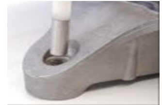
Figure 1 - Eddy Current Thread Probe with SS Sleeve
