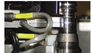
Figure 2 – Eddy Current Probe Details
