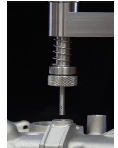
Figure 1 - Spring Loaded Eddy Current Thread Probe
