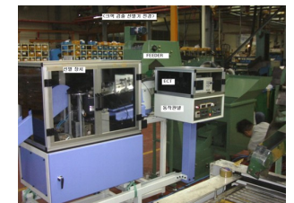
Figure 3 – Production view of eddy current test station
