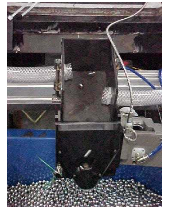
Figure 2 - Eddy current ball bearing test fixture
