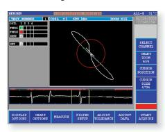
By placing the new coil just after the laser welding operation, the eddy current equipment is capable of detecting bad welds or non-welded areas on the tubing in addition to cracks.
