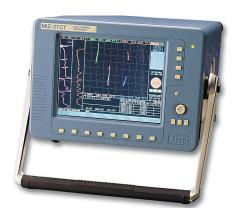
MIZ®-27CT to operate its multi-coil array and collect inspection data. Ceramic rollers guide the product through the probe center and minimize lift-off signals. Custom designed springloaded sled assemblies were built to follow the material undulations rather than force it to conform to a fixed position and risk possible product damage.
