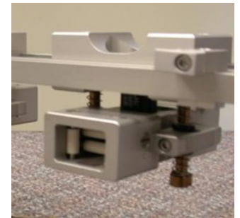
Figure 2 – Eddy Current Probe with Ceramic Guide Rollers
